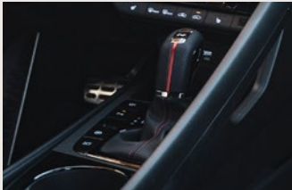
Available N 8-speed Dual Clutch Transmission (N DCT) The N DCT is an automated manual transmission with two separate clutches for increased efficiency, faster shifting and driving convenience.
